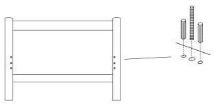
Making the bed. (Two people required) Slide each mattress rail onto the threaded bar and wooden dowels that you have fitted in the legs. Carefully slide the lunar washer onto the threaded bar as it passes through the large hole in each mattress rail. As this bar passes through the lunar washer slip on the spring washer then the normal washer and then finally the nut. Push the bed frame together. Rotate the nut using the spanner provided and tighten the bed frame.
